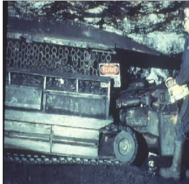
Figure 6. A Mobile Roof Support.
