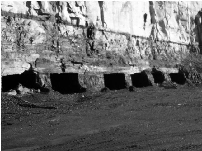
Figure 8. Typical highwall mining web and barrier pillars.
