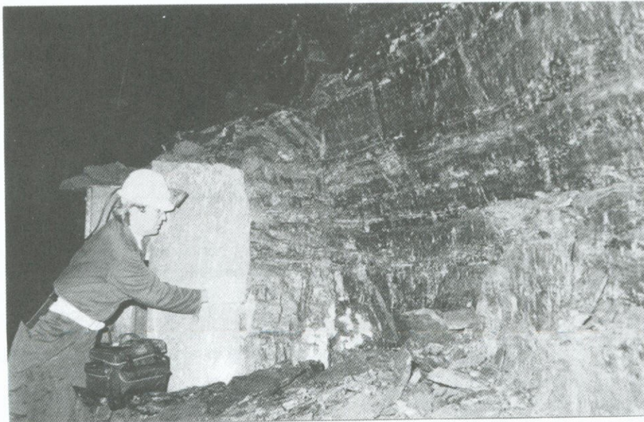
Figure 2. Illustration of progressive pillar scaling.
