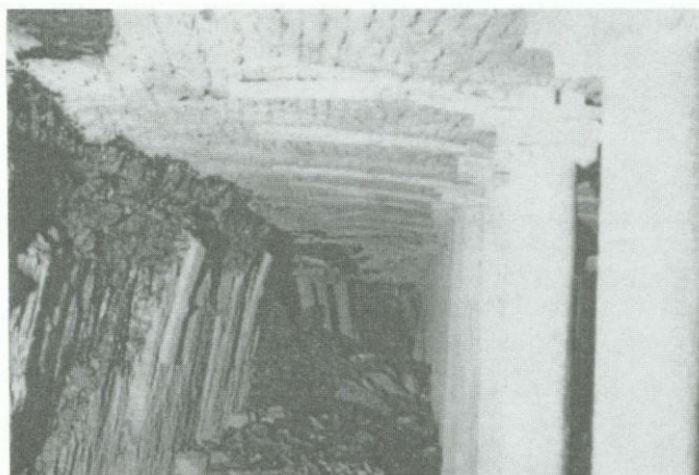
Figure 12c. First open cross cut intersection inby the face supported with Propsetter supports.
