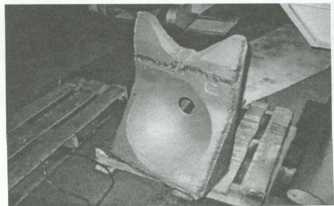
Figure 17. "Zipper-shaped" leg cylinder casting to avoid stress concentration caused by orientation of casting to principal stress field.
