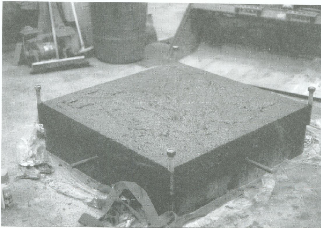
Figure 3. Box frame after loading with loose rock and spray coating with Tekflex.
