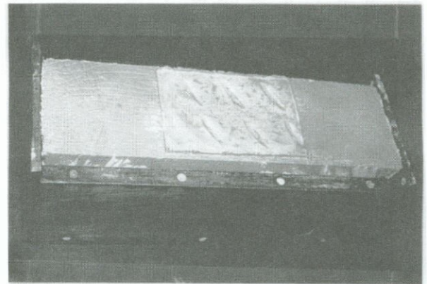
Figure 6: Photograph showing cast resin samples inside the bottom shear box
