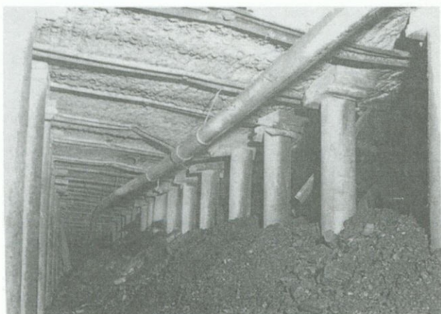
Figure 12b. Inby area supported by Propsetter support.
