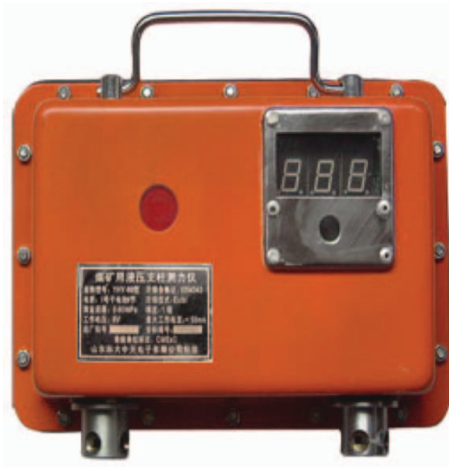
Figure 5. Model KBJ-60-1 continuous pressure recorder.
