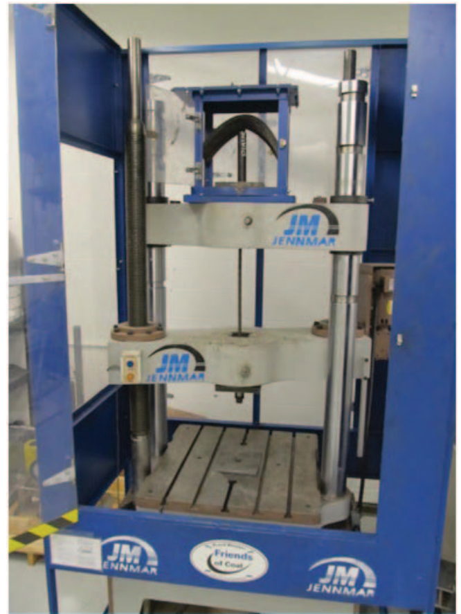
Figure 3. Tensile test of plain cable sample with 12" of resin encapsulation.
