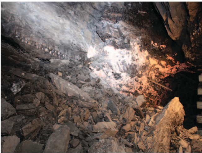
Figure 22. Minor flushing, and excellent gob control.
