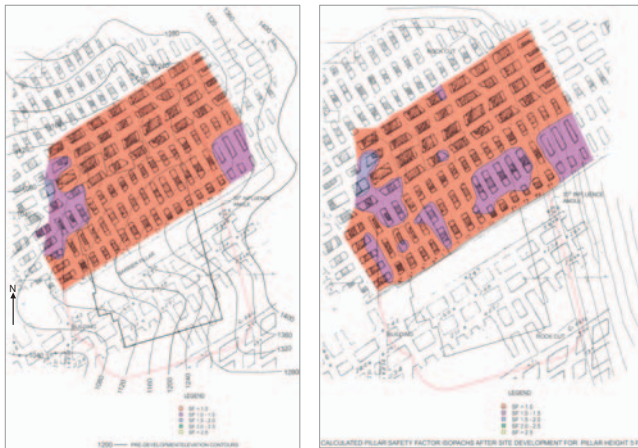
Figure 1. Calculated pillar safety factor isopachs of Mine No. 15 JR below the northern half of the building at the time of second mining (left figure) and after the site development (right figure).
