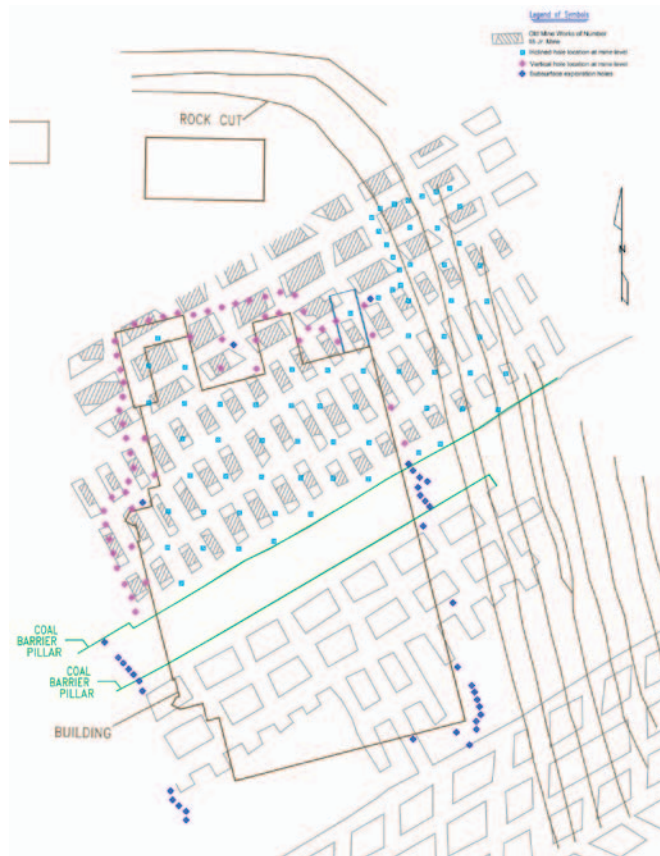
Figure 4. Grout hole location in the northern side of the coal barrier pillar.
