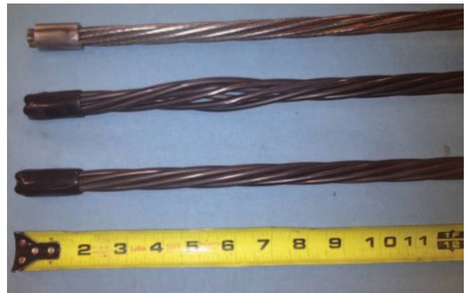
Figure 1. Test Samples, top to bottom: indented cable, plain cable with a single bird cage and plain cable.
