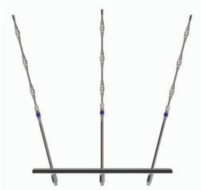
Figure 6. B-Rigid truss system detailing angled cable bolts.
