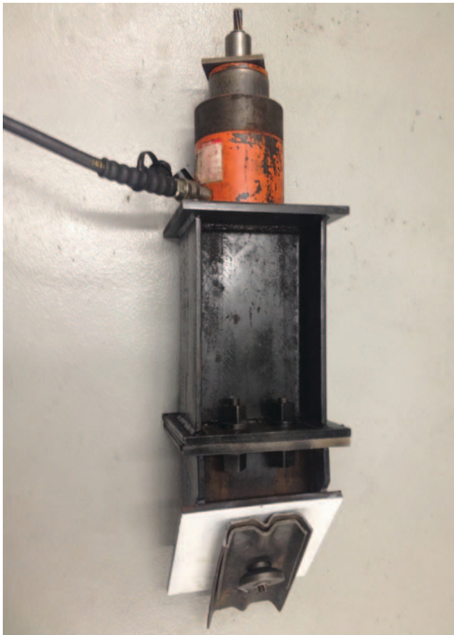
Figure 7. The Off-Axis test fixture allows cable to be aligned at 30 or 45 degrees as load is applied.
