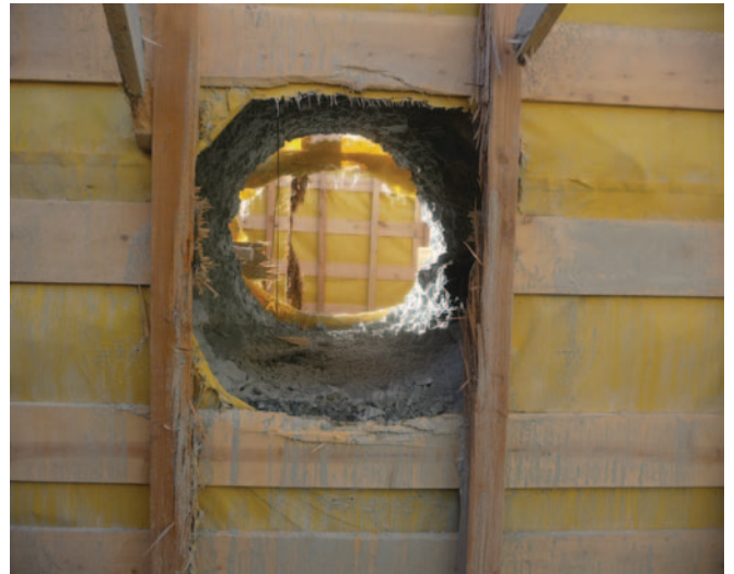
Figure 10. Test breaching 50 psi (0.34 MPa) seal.
