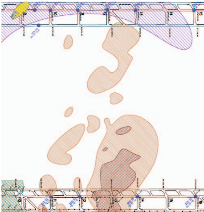
Figure 3. Thick draw slate and advance rates in Panel 15.
