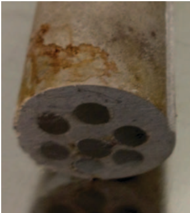
Figure 9. Sectioned bore tube sample of single birdcage sample with clockwise rotation (sample was cut at the birdcage).
