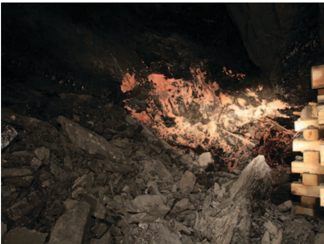
Figure 23. Minor flushing, and excellent gob control.
