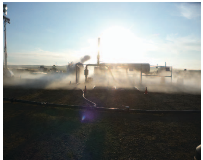
Figure 1. Nitrogen injection on gob vent borehole.
