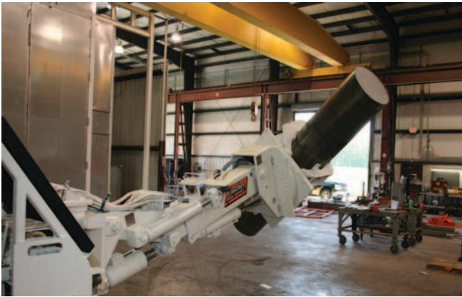
Figure 4. Testing manipulator ability to hold Can support in any position.
