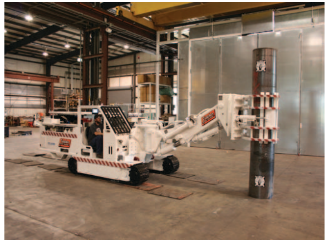
Figure 3. Operator located on right side of machine for enhance visibility.
