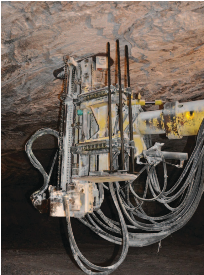
Figure 7. Fully automated drill rig.
