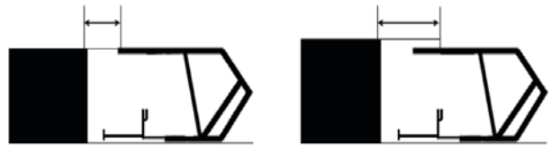
Figure 2. Illustration of the impact of 'steps' in the roof on effective tip to face distance.
