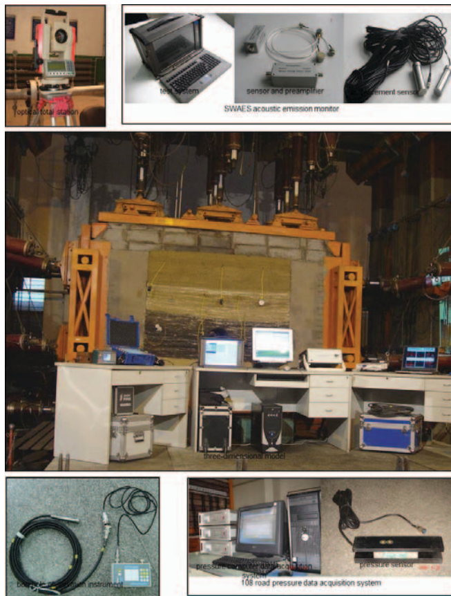
Figure 1. Deformation monitoring system of roadway.
